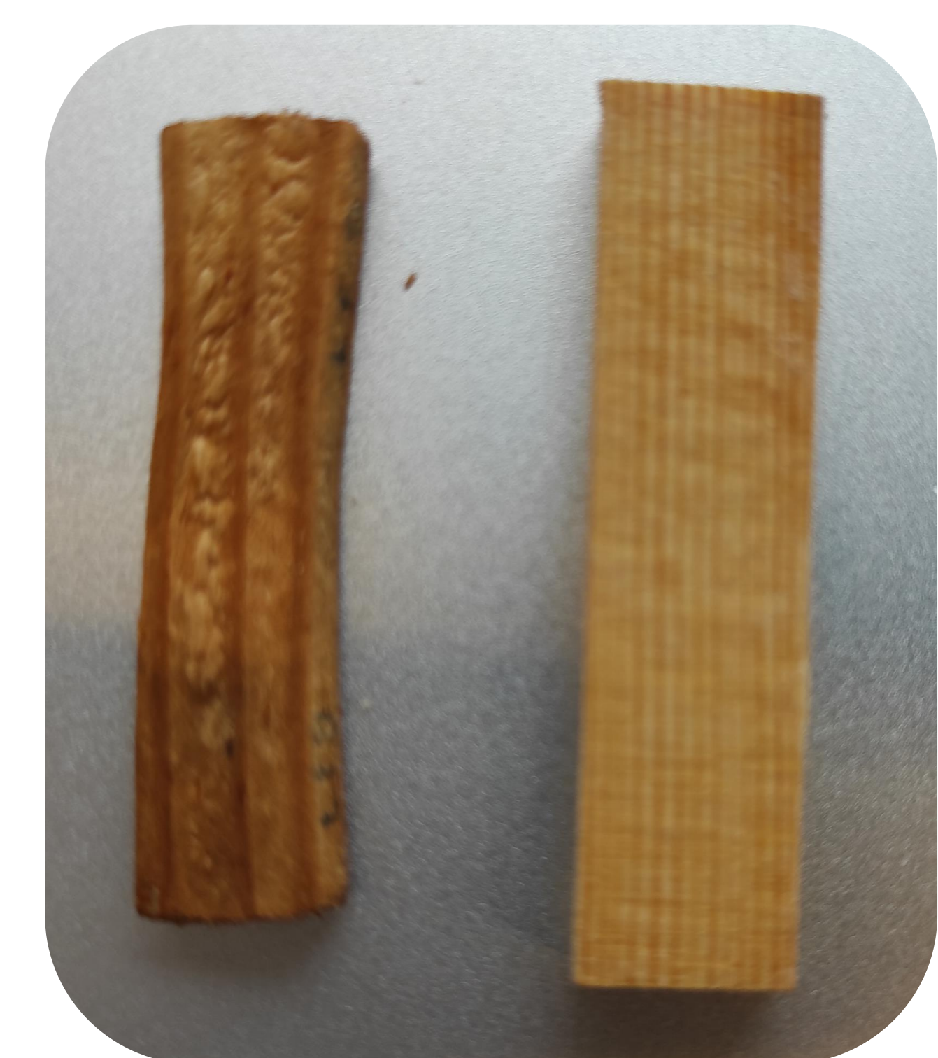
Comparison of control (left) and caffeine-treated (right) wood after 16 weeks of exposure to decay.
